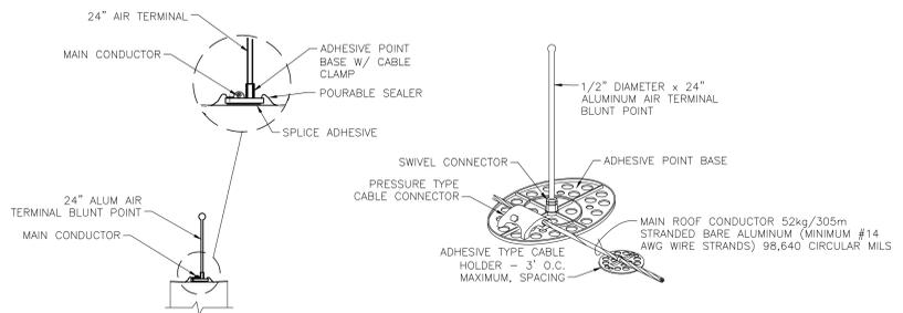
**1 AIR TERMINAL "A" INSTALLATION DETAIL**
