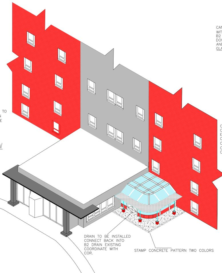
CANOPY TO BE SLOPE WITH 1/8% GRADE BACK TO B2 FOR WATER DRAINAGE. DOWNSPOUT TO BE ATTACHED AND WATER DISCHARGED AWAY FROM GLASS STRUCTURE AND B2.
