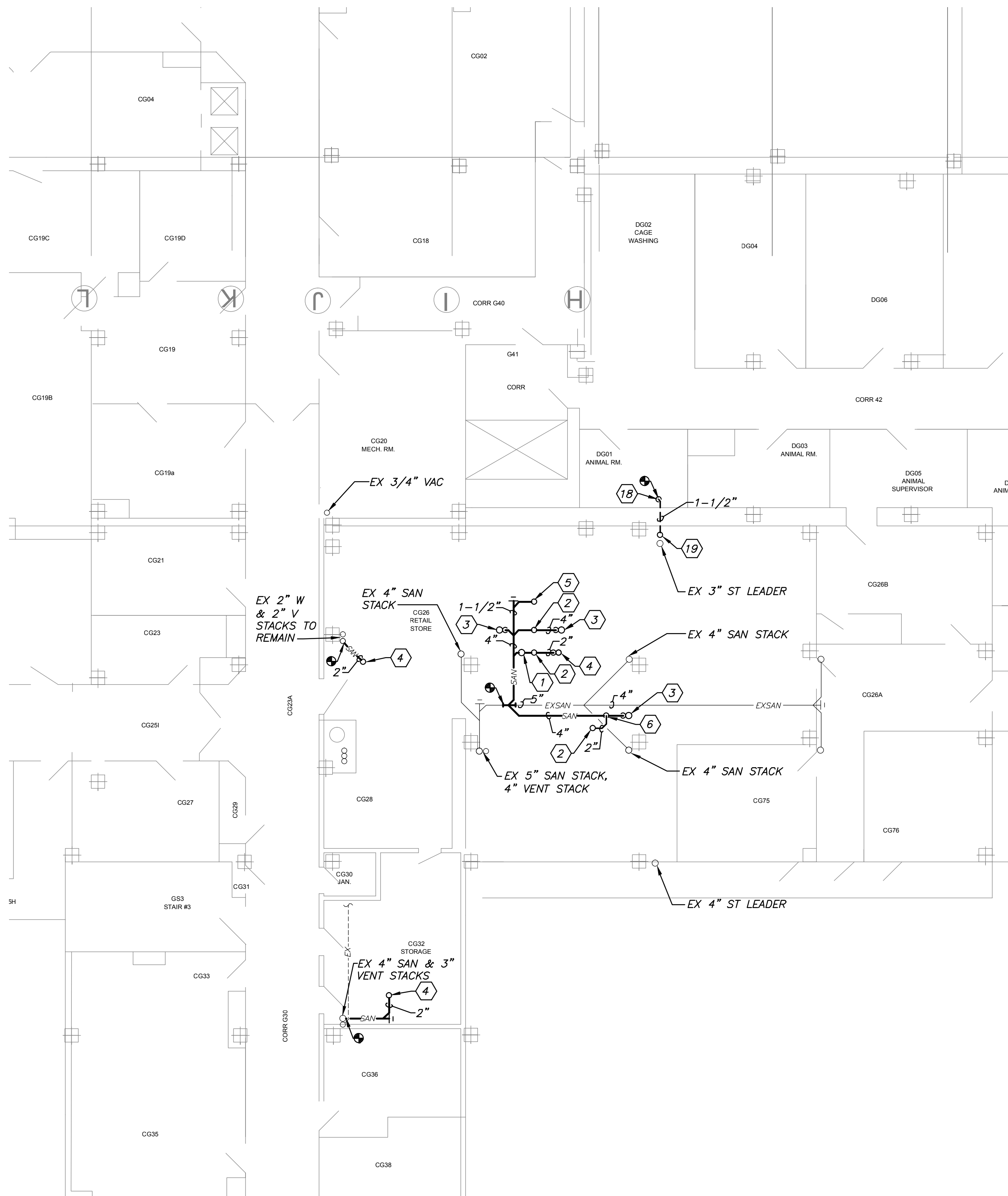
2 P1 GROUND FLOOR PLUMBING PLAN - DRAINAGE SCALE: 1/8" = 1'-0"
