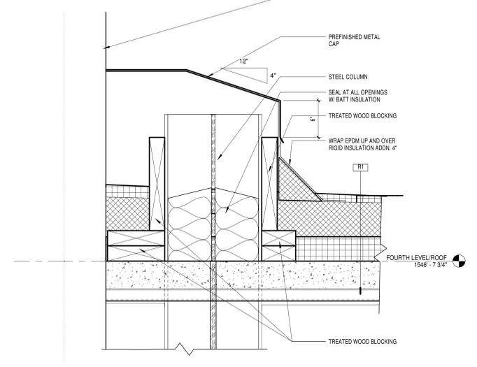
**8B STEEL COLUMN THROUGH ROOF & COLUMN COVER**
