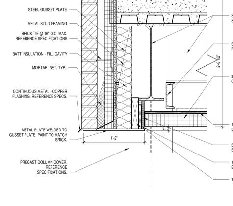
**3E EXTERIOR DETAIL @ SOFFIT**
