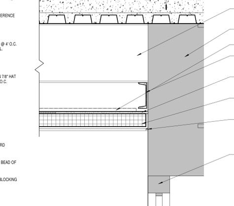
**7E SOFFIT DETAIL AT FACE OF WALL**
