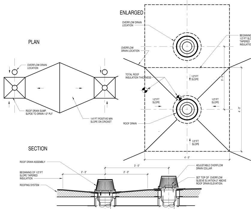
**1C ROOF DRAIN AND OVERFLOW DRAIN DETAILS**
