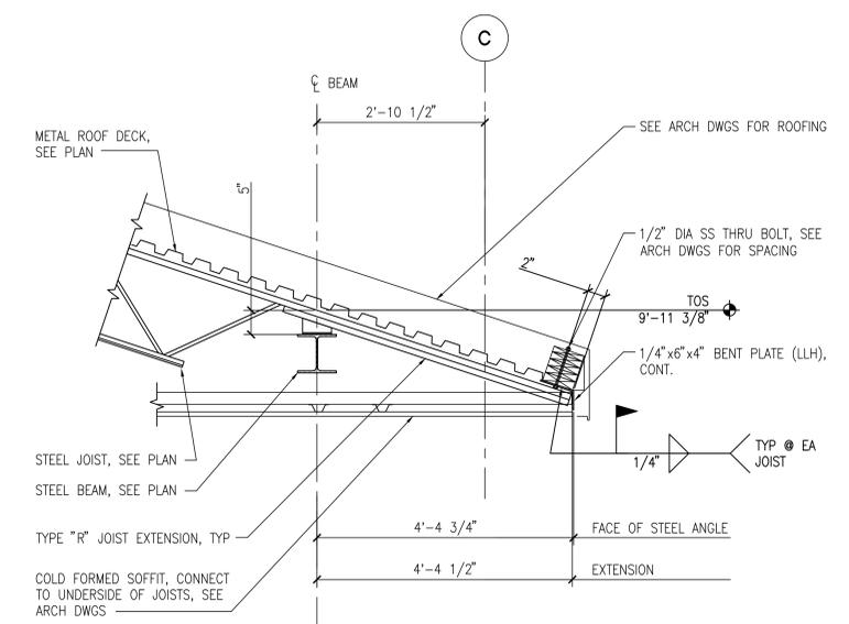
3 ROOF SECTION AT LOADING DOCK WALL
