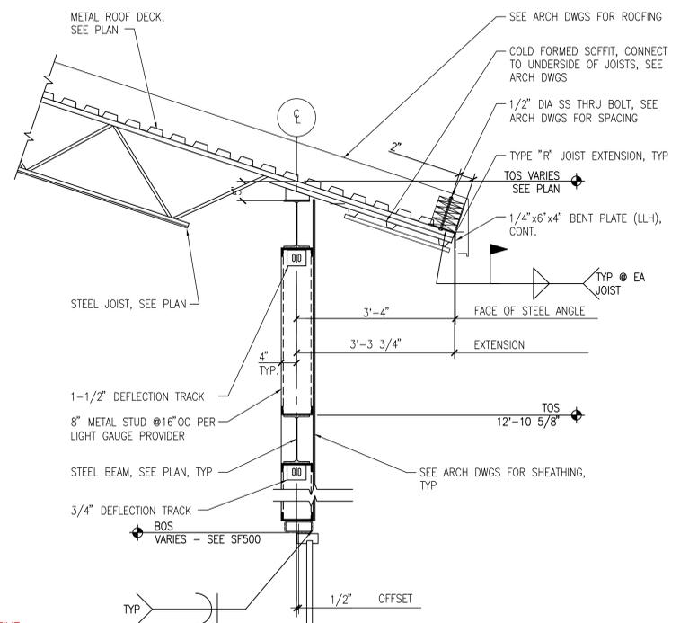
2 ROOF SECTION AT EXTERIOR WALL - FRAMES #5, #9
