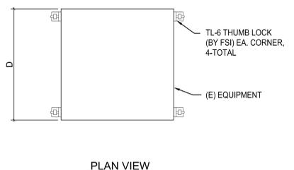
9 WITH-LEGS COUNTER MOUNTED EQUIPMENT ANCHORAGE
