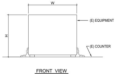
5 EQUIPMENT WALL ANCHORAGE - WITH METAL TOP
