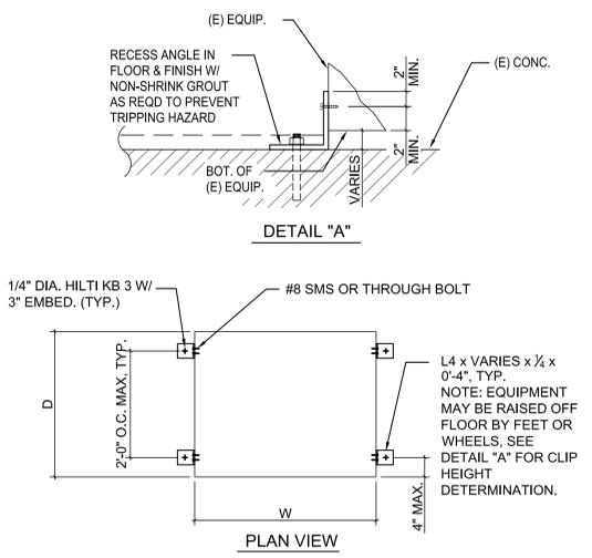
3 TYPICAL ANCHORAGE FOR EQUIPMENT ON FLOOR
