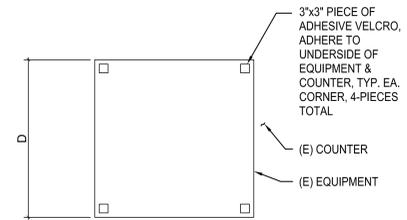
7 LEG LESS COUNTER MOUNTED EQUIPMENT ANCHORAGE
