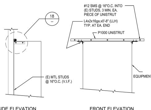
12 EQUIPMENT WALL ANCHORAGE - NO METAL TOP
