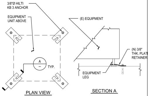
13 LEG ANCHORAGE FOR FLOOR MOUNTED EQUIPMENT
