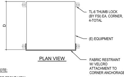
10 WITH-LEGS COUNTER MOUNTED EQUIPMENT ANCHORAGE
