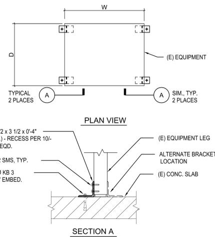
1 LEG ANCHORAGE FOR FLOOR MOUNTED EQUIPMENT
