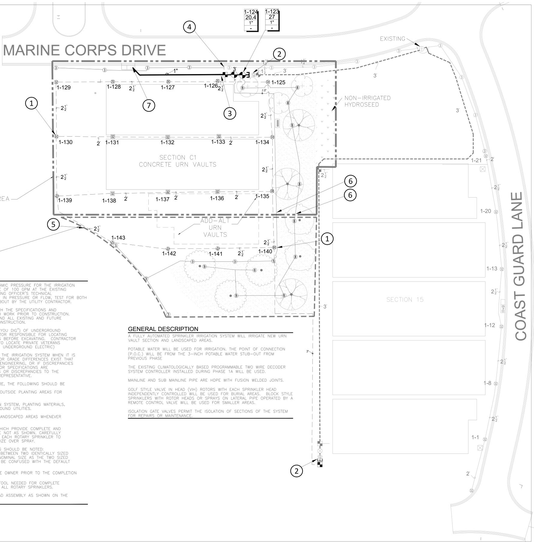
ADD-ALTERNATE #1 LIMIT OF WORK OVERLAPS INTO BASE BID AREA FOR GRADING AND URN VAULT INSTALLATION. PLANTING AND IRRIGATION WORK DOES NOT OVERLAP
