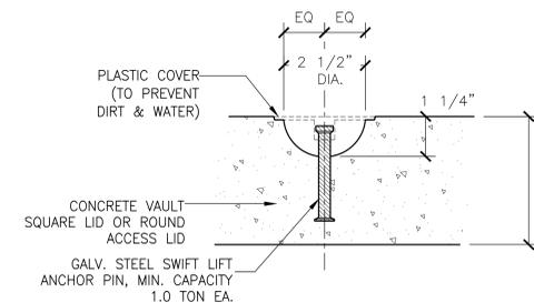
**B8** 1-TON SWIFT LIFT ANCHOR - SECTION DETAIL
